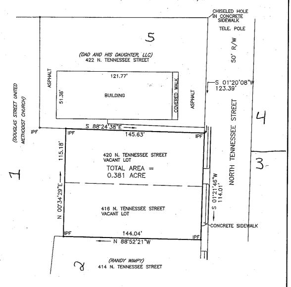
FIELD TRAVERSE: CLOSURE; ONE FOOT IN 20,000 FEET USING A LIETZ SET 3. ANGULAR ERROR; 0'00'06"PER ANGLE POINT USING A LIETZ SET 3. ADJUSTED; USING THE COMPASS RULE.
