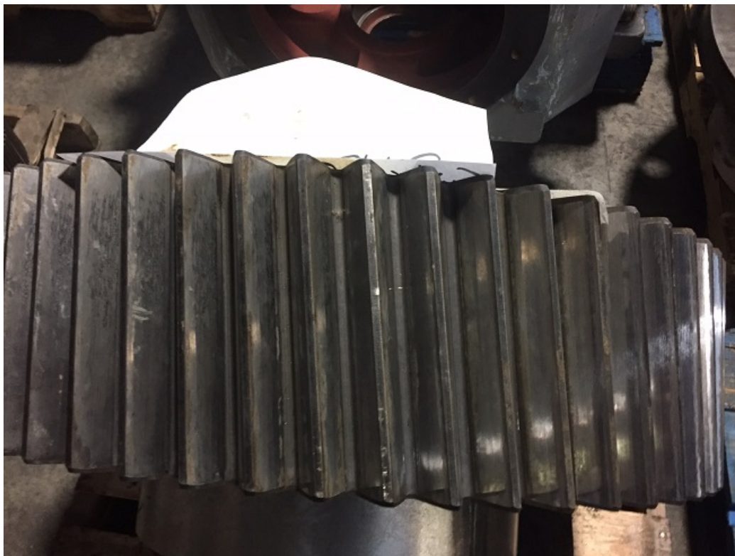
Low-speed gear teeth in good condition
