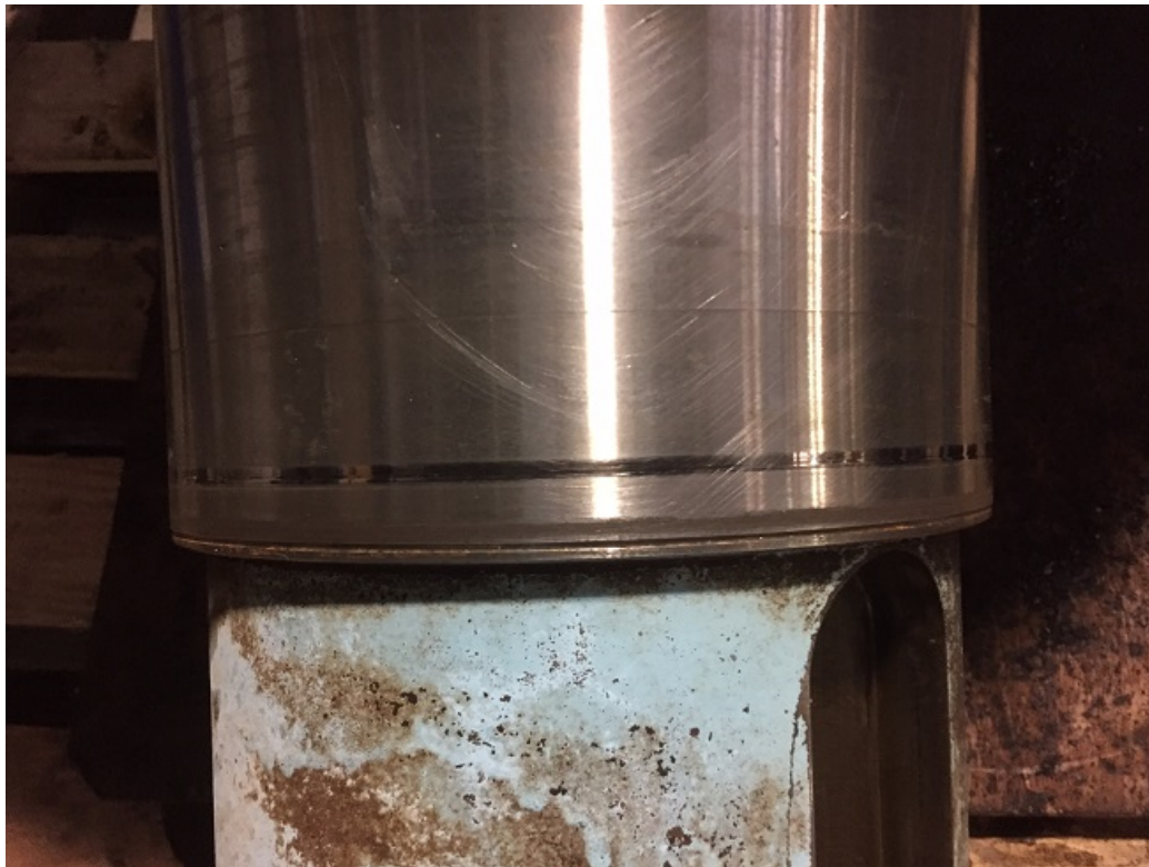
Output Seal Area requiring repair
