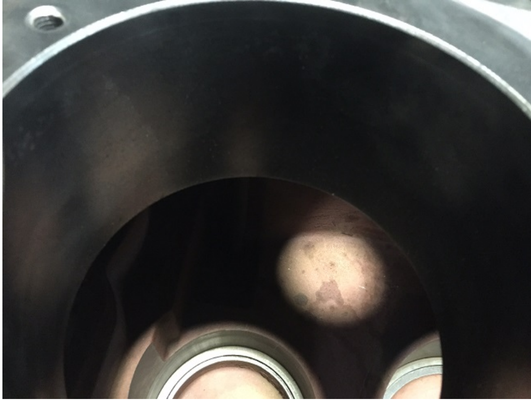
Damaged 2 nd reduction pinion bore
