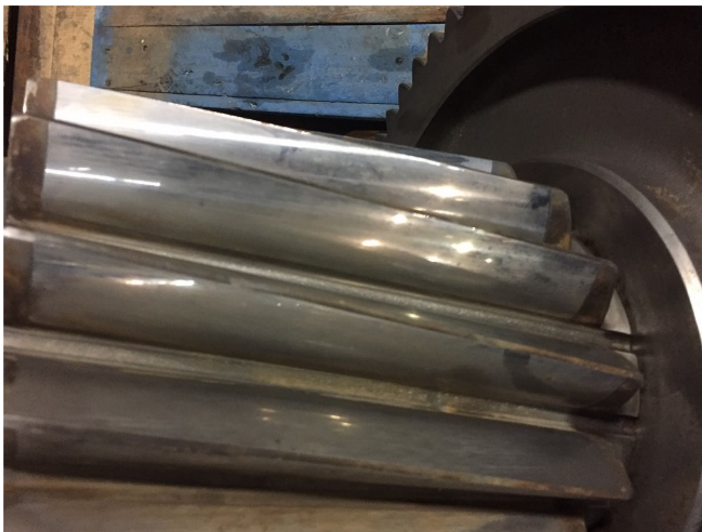
Low-speed Pinion teeth in good condition
