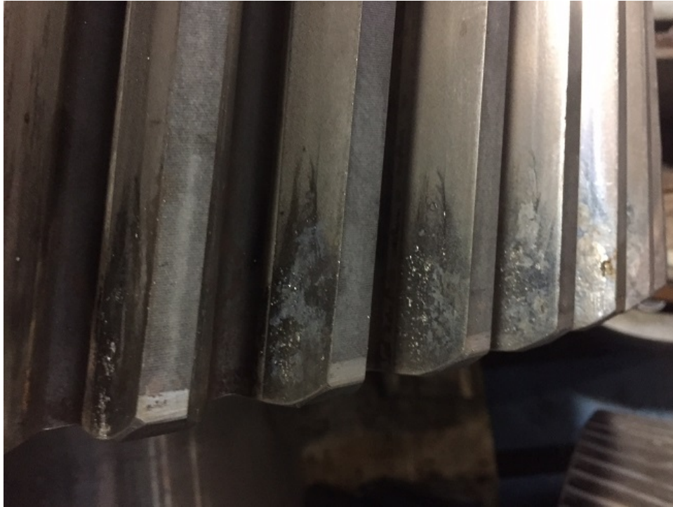
Heavily worn and pitted Low-speed gear
