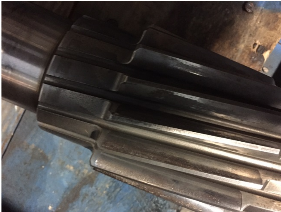
Worn High-speed pinion
