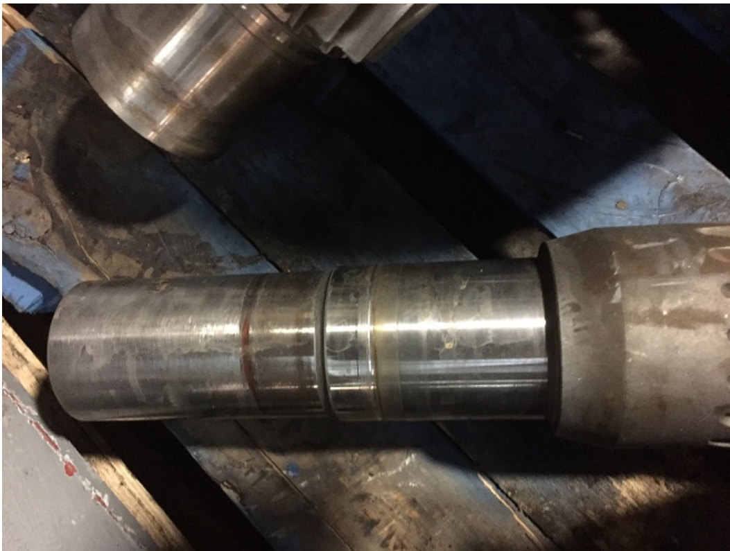
Input Seal Area requiring repair
