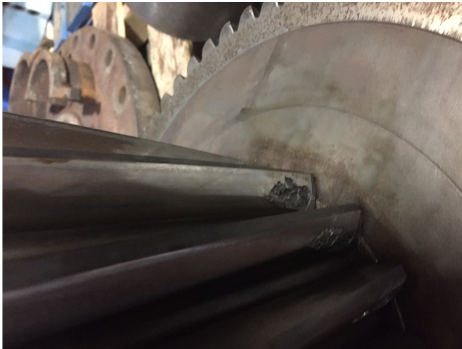
Damaged Low-speed Pinion
